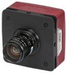
Click to Enlarge USB Camera with MVL25M23 C-Mount Camera Lens
